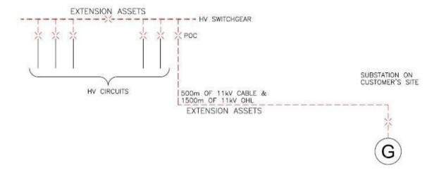
The existing switchgear had fault level rating of 250MVA. The company no longer uses switchgear with a fault level rating of 250MVA, so uses the closest equivalent switchgear used by it as standard, which has a slightly higher rating. Whilst the replacement switchgear increases the fault level capacity and
