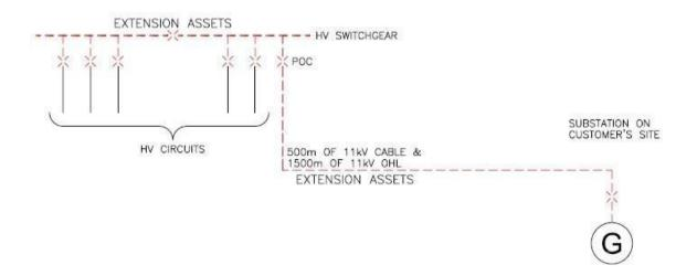
The existing switchgear had fault level rating of 250MVA. The company no longer uses switchgear with a fault level rating of 250MVA, so uses the closest equivalent switchgear used by it as standard, which has a slightly higher rating. Whilst the replacement switchgear increases the fault level capacity and
