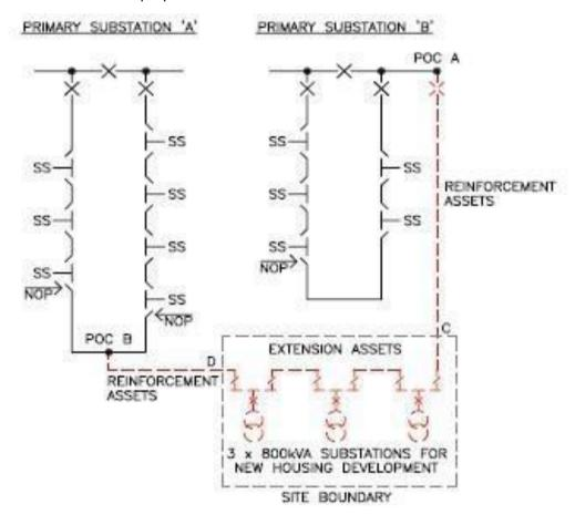
The assets connecting Point of Connection A and Point of Connection B add capacity to the existing network, so would normally be treated as Reinforcement. These comprise:
